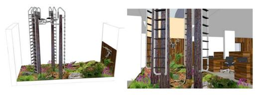
This project called 'RESERVOIR' is a combination of a green roof and a green courtyard. On the bottom it creates a forest ground by using a high volume of leaves which will – over time – transform into soil and allow plants to grow from the seed reservoir held in the material. The sculptural elements are designed a hybrid objects between Trees, lookouts and pool ladders. They symbolise communication, observation, expansion and positively irritate by their ambiguous meaning.
